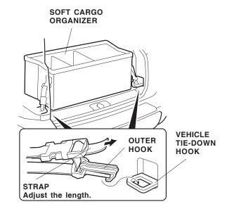
4. Adjust the length of the strap as needed to secure the organizer to the tie-down hooks.
