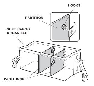
3. Place the organizer in the cargo area of the vehicle. Attach the outer hooks of the organizer to the vehicle tie-down hooks.
